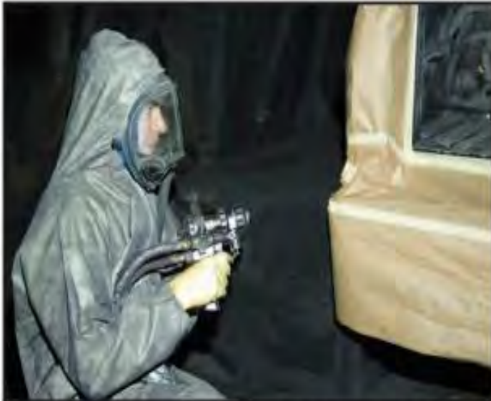
Worker applying spray-on polyurethane truck bed liner Source: Wikimedia / Creative Commons
